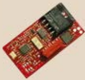
RF UNI with filter 433 - 868 MHz
